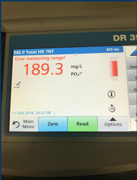
Figure 12: Phosphate Reading Factor of 10 Photo courtesy of Cameron Rhodes
