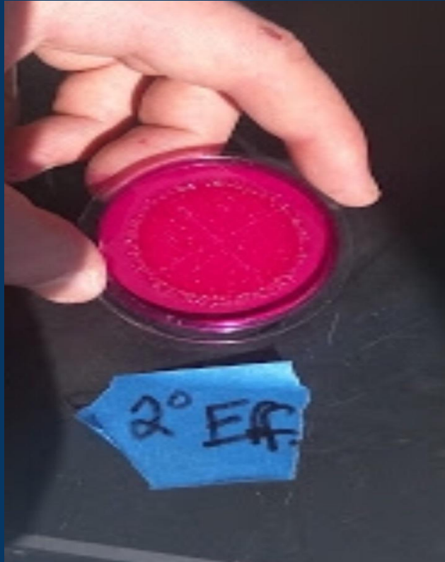
Figure 4: Secondary Effluent for Total Coliforms Results Photo courtesy of Cameron Rhodes
